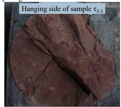
(l) failure plane of rock mass under 2.1 MPa normal stress: concrete covering effect
