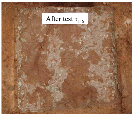
(c) rock mass after shear test: no surface effect
