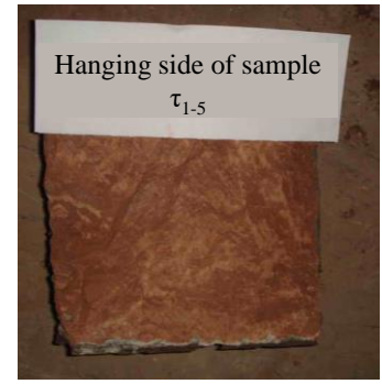
(c) failure plane of rock mass under 1.5 MPa normal stress: no surface effect
