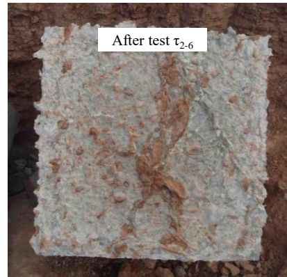
(l) concrete side after shear test: dry-wet cycling effect
