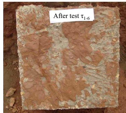
(d) concrete side after shear test: no surface effect
