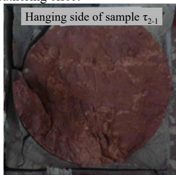
(h) failure plane of rock mass under 0.4 MPa normal stress: dry-wet cycling effect
