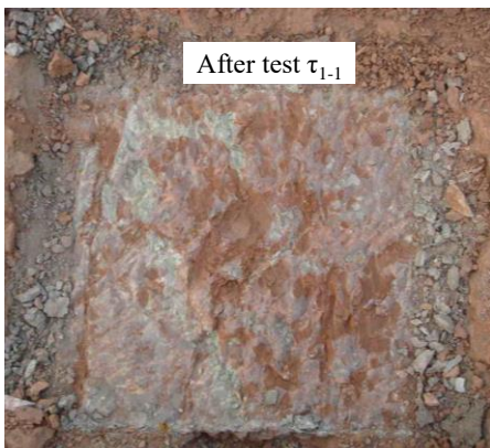
(g) rock mass side after shear test: natural weathering effect
