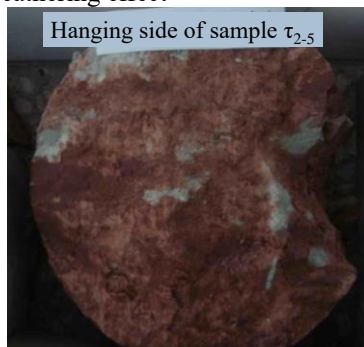
(i) failure plane of rock mass under 2.1 MPa normal stress: dry-wet cycling effect
