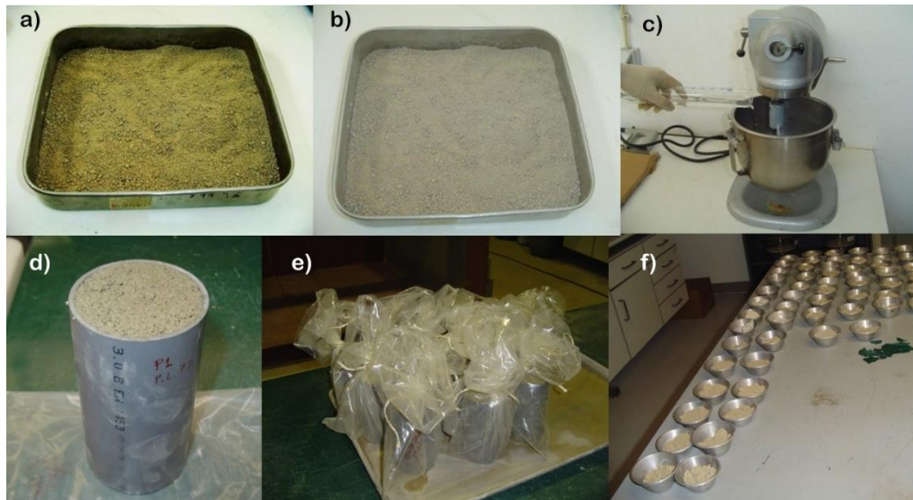
Fig. 2 (a) soil, (b) soil homogenized with cement, (c) addition of water using a mixer, (d) fresh test specimen, (e) bagged fresh test specimens and (f) portions to determine water content
