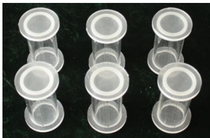
Fig. 3 Molds for standard reinforced cylinder sample
