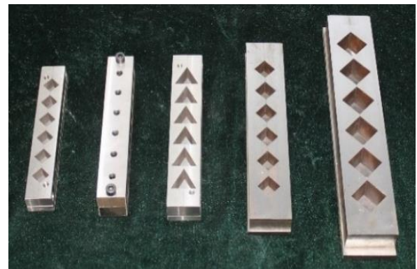
Fig. 2 Molds for mortar specimens
