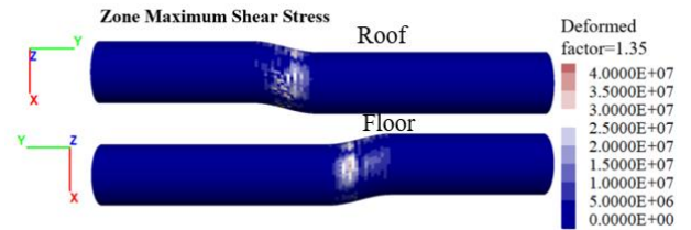
Fig. 21 Calculated maximum shear stress contour on roof and bottom of tunnel (unit in Pa)
