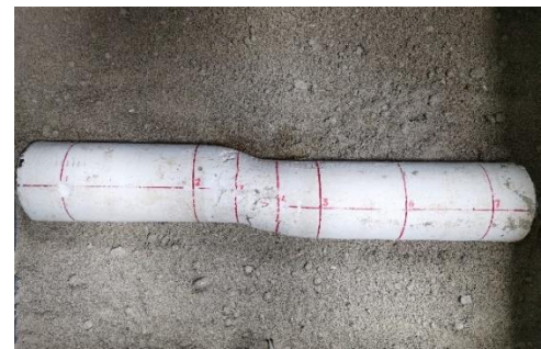
Fig. 13 The deformed tunnel model after test
