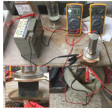
Fig. 5 Electrical resistivity test set-up
