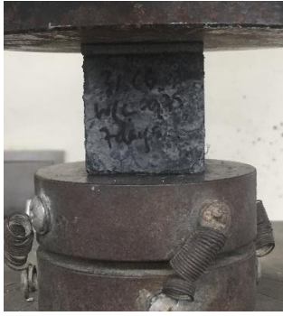
Fig. 6 Typical compression testing of a stabilized specimen
