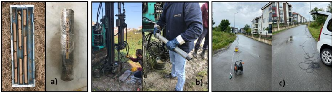
Fig. 6 (a) UD sample, (b) SPT tests and (c) Vs tests
