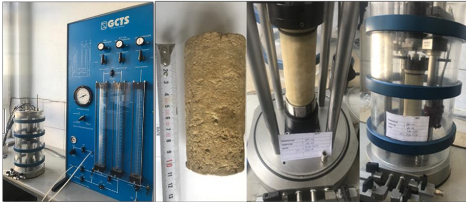
Fig. 13 Undisturbed sample and resonant column test system
