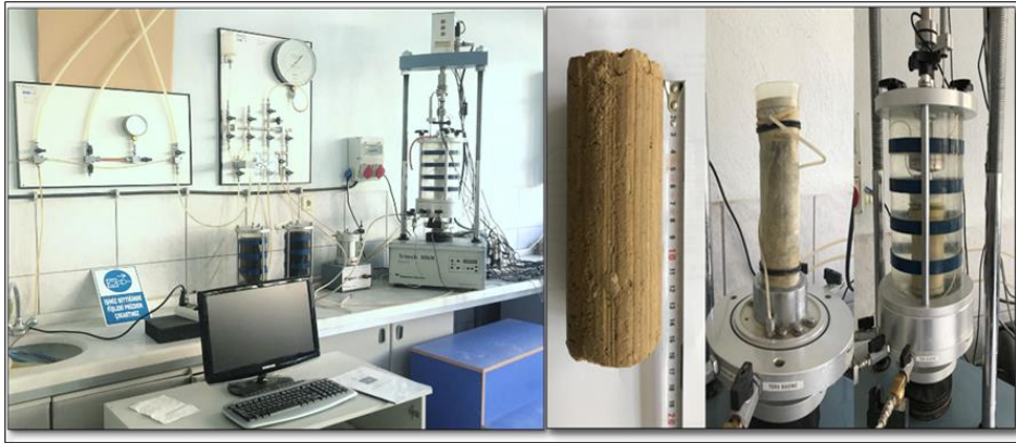
Fig. 12 Undisturbed sample and dynamic triaxial test system
