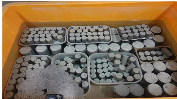
Fig. 7 Water curing specimens(3, 7, 15, 28 days)
