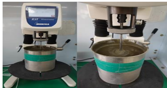
Fig. 6 Viscosity measurement using rheometer SST
