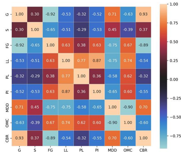
Fig. 2 The correlation between CBR values and soil parameters
