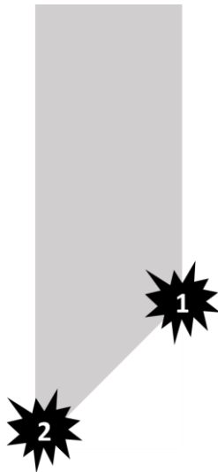
Fig. 8 Location of the maximum stress concentration
