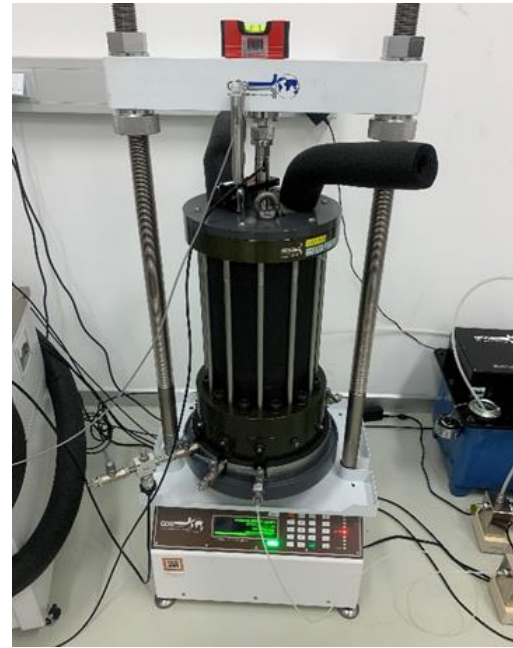
Fig. 3 GDS Triaxial Automated System: (a) Schematic diagram and (b) Photograph of the high-pressure triaxial cell in the loading frame
