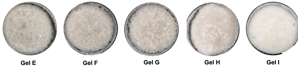
Fig. 7 CaNaXS Gel uniformity with various crosslinker ratios
