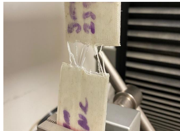
(b) Separation and deformation of layers after the failure
