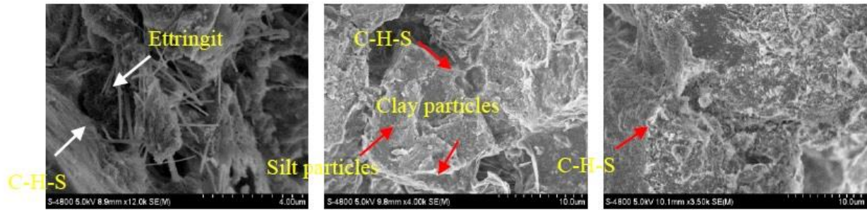
(d) Hydration products of hydrated lime and GGBFS (e) Content of 3% curing agent (Active MgO) (f) Content of 15% curing agent (Active MgO)
