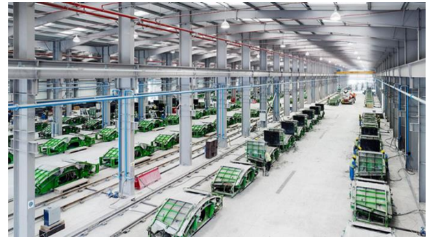
Fig. 1 Segment factory with Static Moulds
