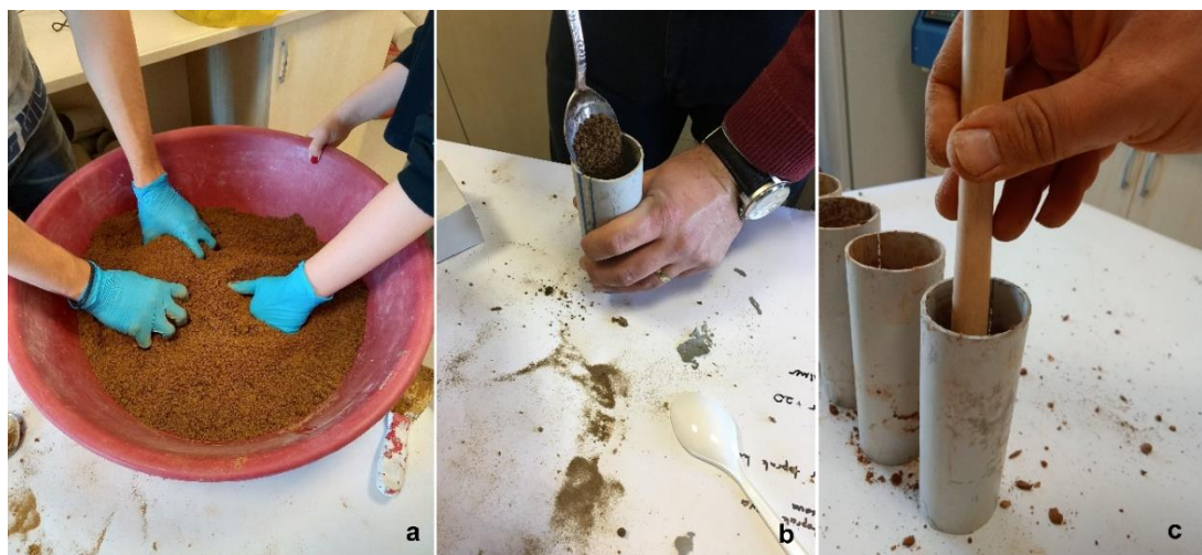
Fig. 3 (a) Soil mixing, (b) soil moulding and (c) soil compaction in moulds
