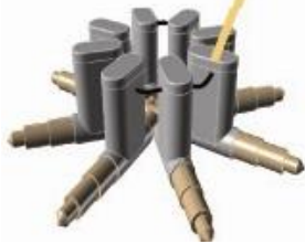
Fig. 9 Application of pressure forces by compressor to expand arms
