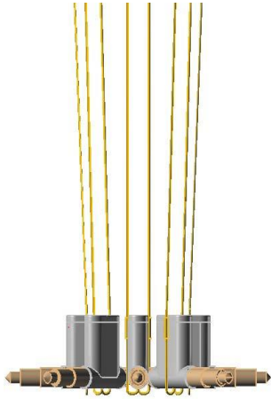
Fig. 8 Application of tension forces through tensile jacks into cables connected to pistons results in opening the arms
