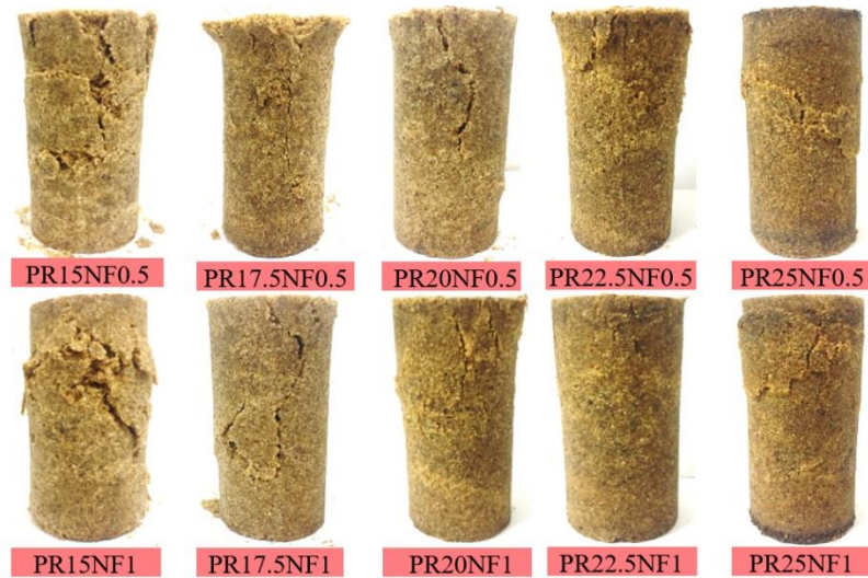
Fig. 5 Compressive failure of the NFRTS
