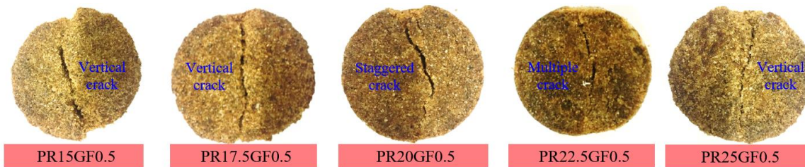
Fig. 10 Failure pattern under splitting tension test of the GFRTS
