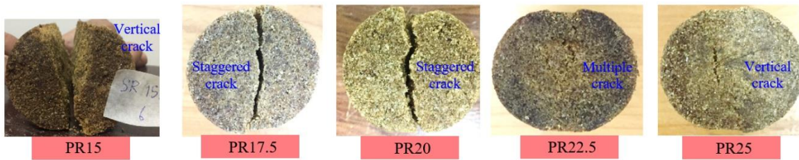
Fig. 8 Failure pattern under splitting tension test of the PRTS
