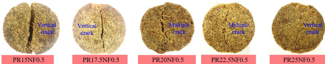
Fig. 9 Failure pattern under splitting tension test of the NFRTS
