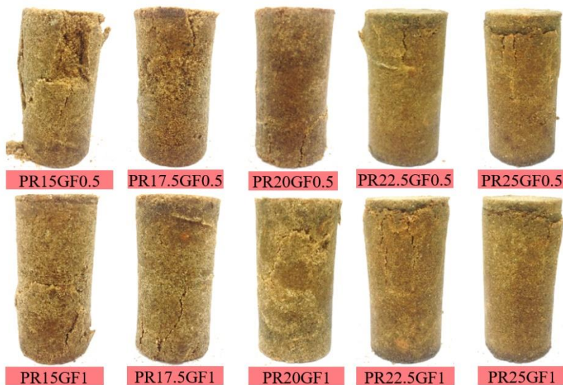
Fig. 6 Compressive failure pattern of the GFRTS
