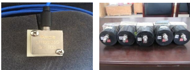
(a) Accelerometers (b) Displacement meters
