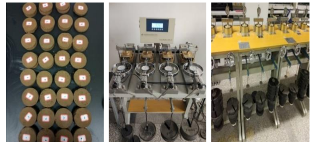
Fig. 5 Indoor direct shear and compaction tests
