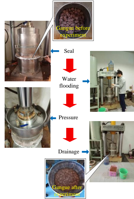
Fig. 5 Crushing gangue compression test in soaking state
