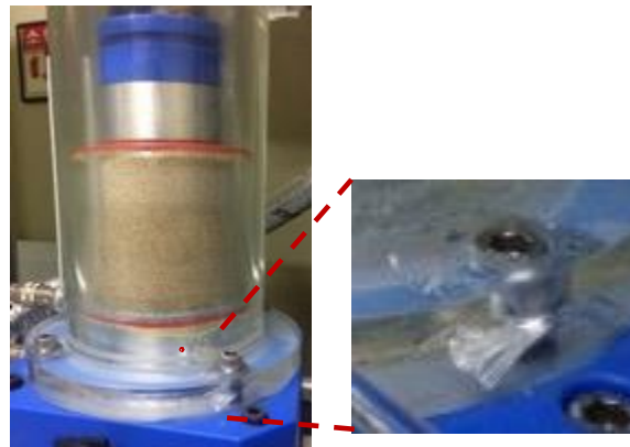
(a) Damage to temperature-controllable cell during downward freezing (Jin et al. , 2019a)
