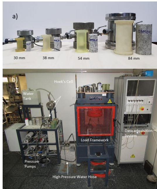
Fig. 1 (a) Different size specimens, sleeves and Hoek's cells to be tested and (b) Testing system and associated elements
