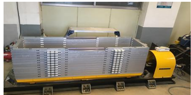
(a) Laminar shear box in this study
