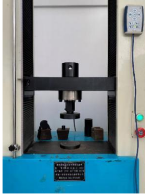
Fig. 7 Computer-controlled rock tensile splitting testing machine
