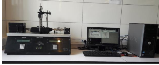
Fig. 3 Geocomp Trac II direct shear test device used in the study
