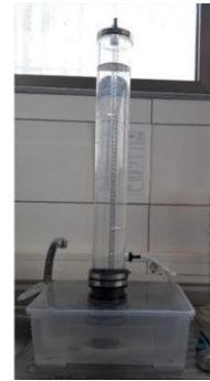
(c) Trautwein bubble tube permeameter
