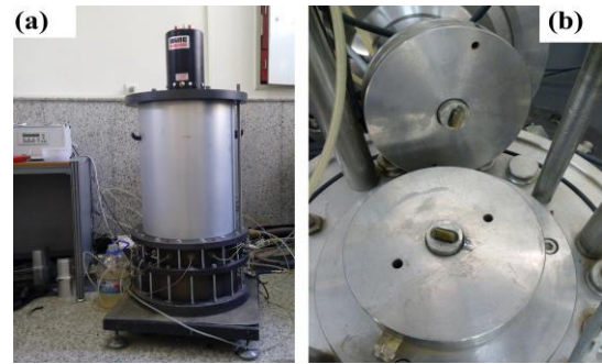
Fig. 1 (a) Resonant column device (b) Bender element setup used for the current study
