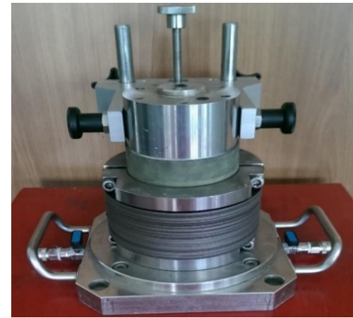
Fig. 2 Dynamic simple shear test apparatus used in the study
