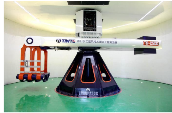
Fig. 1 TK-500 geotechnical centrifuge
