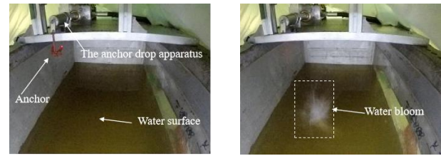
(a) Before anchor drop (b) After anchor drop Fig. 8 Snapshots of anchor drop test in saturated sand
