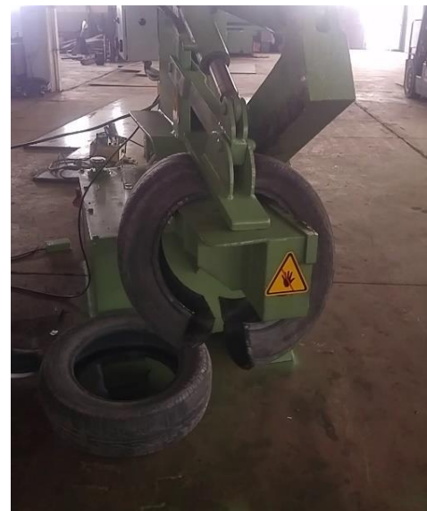
Fig. 2 Waste tire disintegration process
