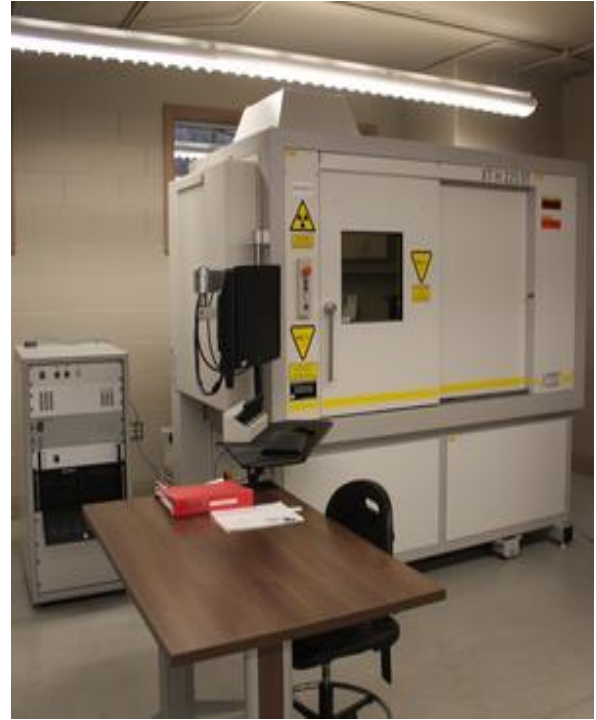
Fig. 3 Micro-CT scanner used for fiber orientation distribution (Located at the Department of Sustainable Archaeology, Western University) (Safdar 2018)
