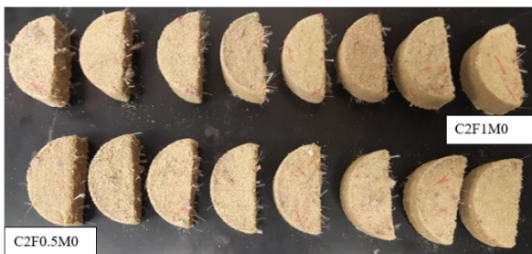
Fig. 5 Vertical and horizontal sections of fiber reinforced cemented Toyoura sand specimens using a thin bench saw (Safdar 2018)
