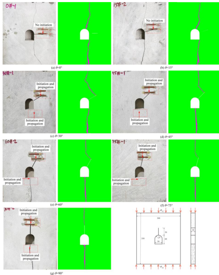
Fig. 12 Comparison of cracking patterns between test results and simulation results under dynamic loads
