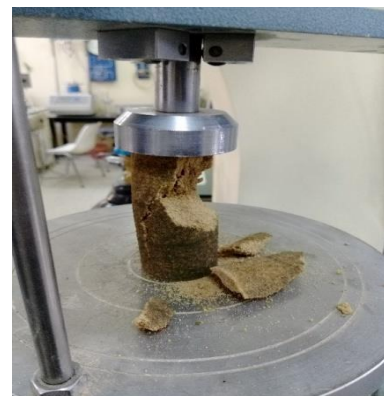
Fig. 4 Unconfined compression test
