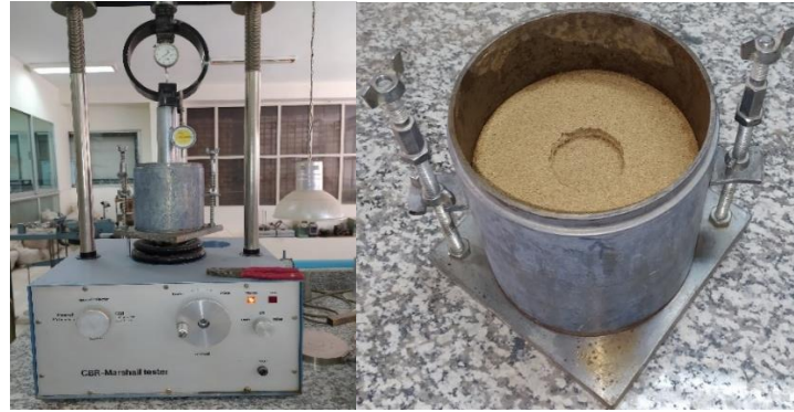
Fig. 5 CBR test on treated sand samples
