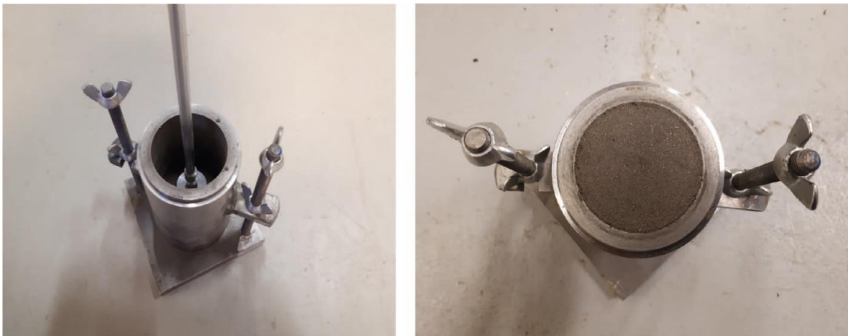
Fig. 3 A manufactured mould (50 × 100 mm) for the under compaction method
