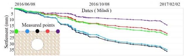
Fig. 4 Cumulative surface settlements at the monitored section
