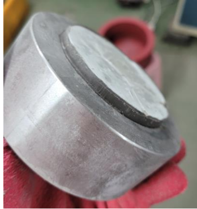
Fig. 7 Field clay-stainless steel ring structure after test
