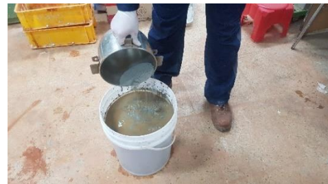
(c) Addition process of cement or cement with GGBS
