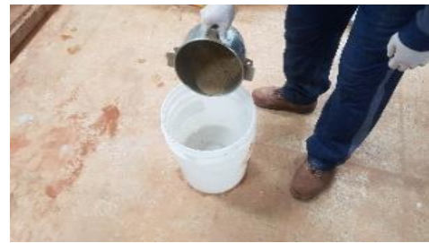
(a) Placement of bentonite with water
