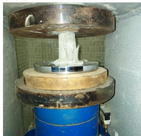
(d) A core prepared from natural cuttings after UCS test
