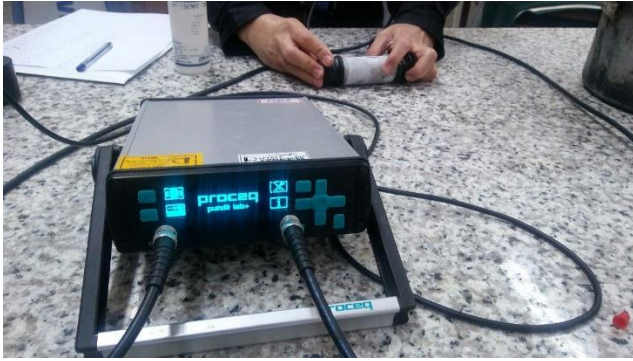
Fig. 1 Vp and Vs measuring device used in this study
