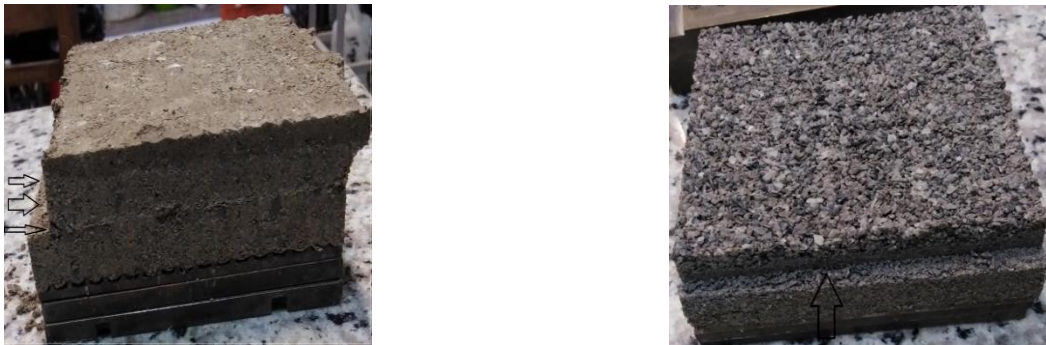
Fig. 13 Sample images after direct shear test (the direction of the arrowheads shows the direction of shear surface): natural cuttings (left side) and artificial cuttings (right side)
