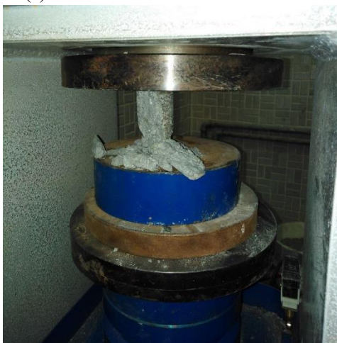
(c) A core prepared from artificial cuttings after UCS tes
