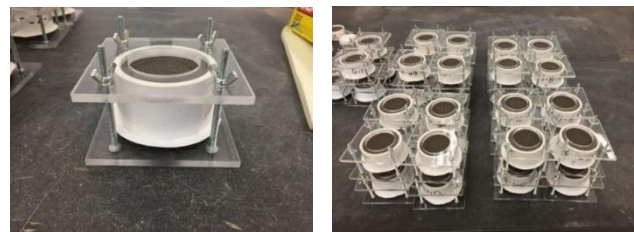
Fig. 6 Samples locked in the mold for weathering
