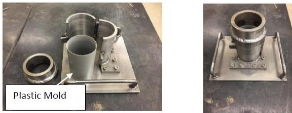
Fig. 3 Plastic mold (PM) for compaction
