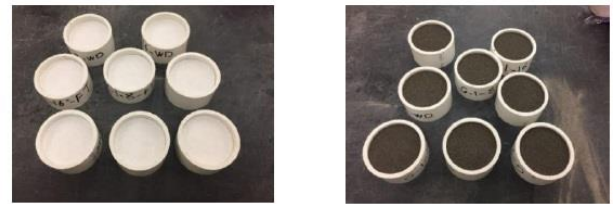
(b) Soil samples with filter paper placed (c) Soil samples with porous stone placed
