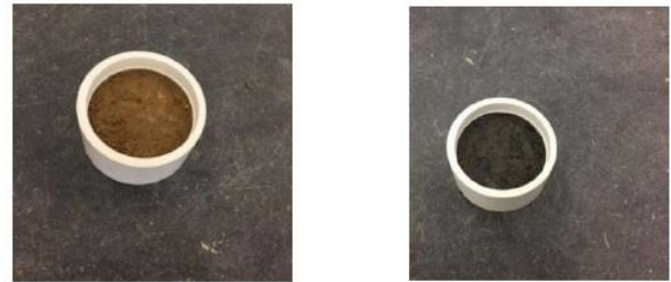
(a) Soil sample in the weathering ring (Left: Glacial Till, Right: Crushed Shale)
