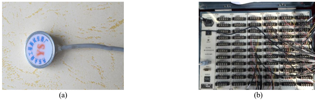
Fig. 9 Stress monitoring system: (a) pressure cell of resistance type and (b) data acquisition system
