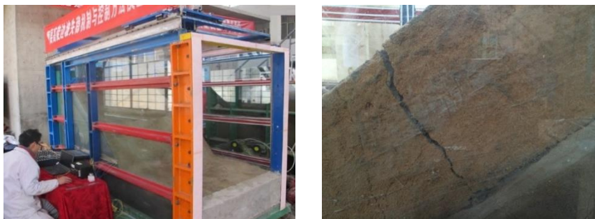
Fig. 14 (a) The overall model test system in the loading process and (b) The typical failure in the loading process.
