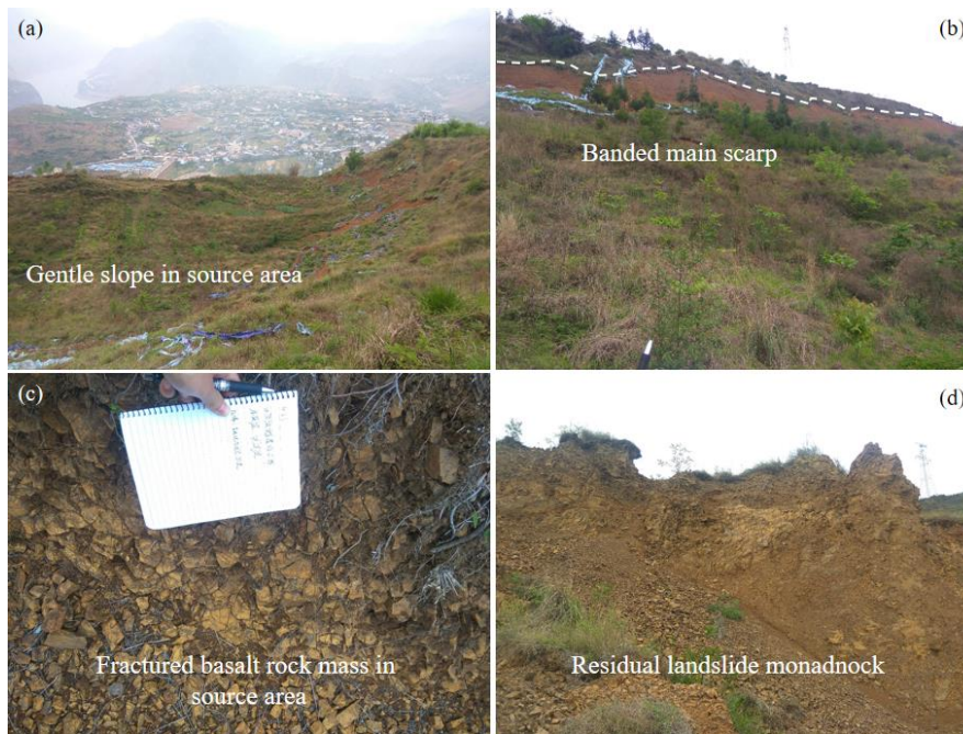
Fig. 6 Characteristic of the source area. (a) Gentle platform formed in the rear edge of source area due to the slow sliding velocity, (b) Banded main scarp in the source area, (c) Fractured rock masses observed in the back wall and (d) Residual landslide monadnock deposited in the source area
