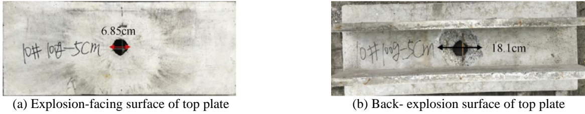
Fig. 5 Damage effect of \pi beam in explosion test under Y1 condition
