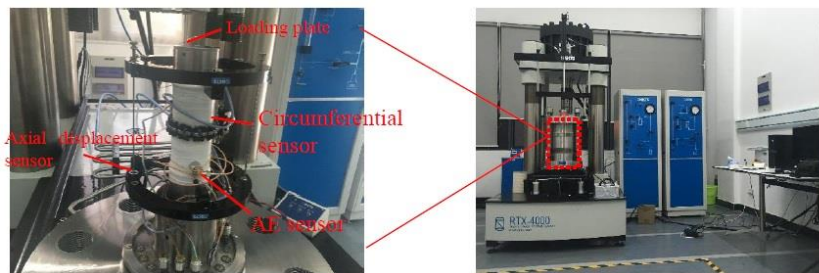
Fig. 3 GCTS RTX-4000 triaxial rock testing system
