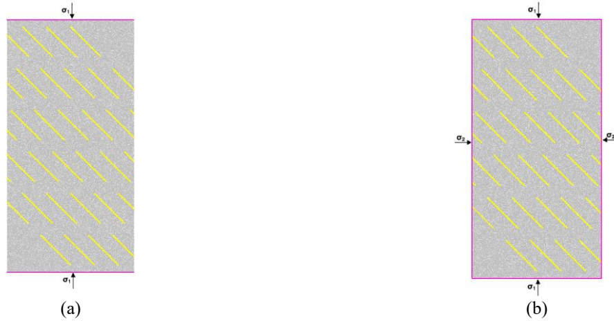
Fig. 10 A typical non-persistent jointed rock mass model (a) Uniaxial compression test and (b) Biaxial compression test
