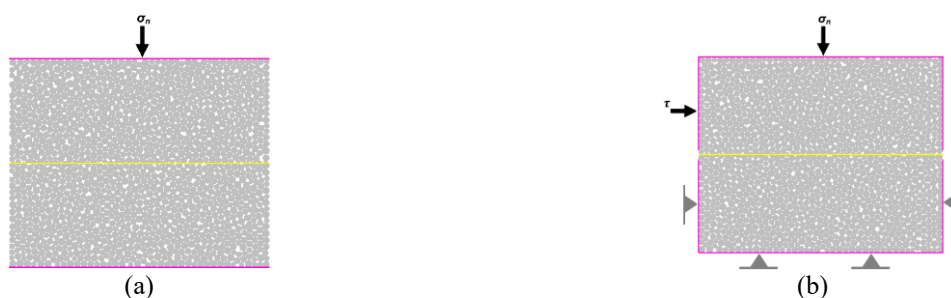
Fig. 8 Numerical experiments to calibration smooth joint parameters (a) Normal deformability test and (b) Direct shear test
