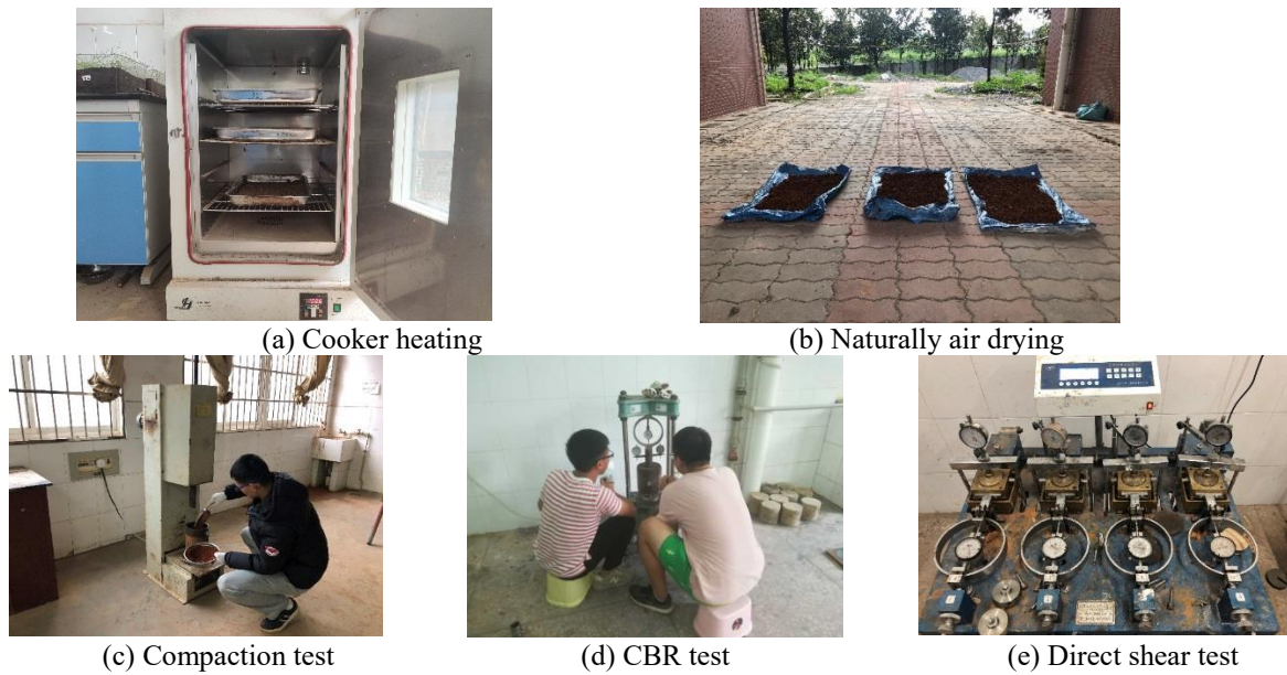
Fig. 2 Specimen forming and mechanical property tests
