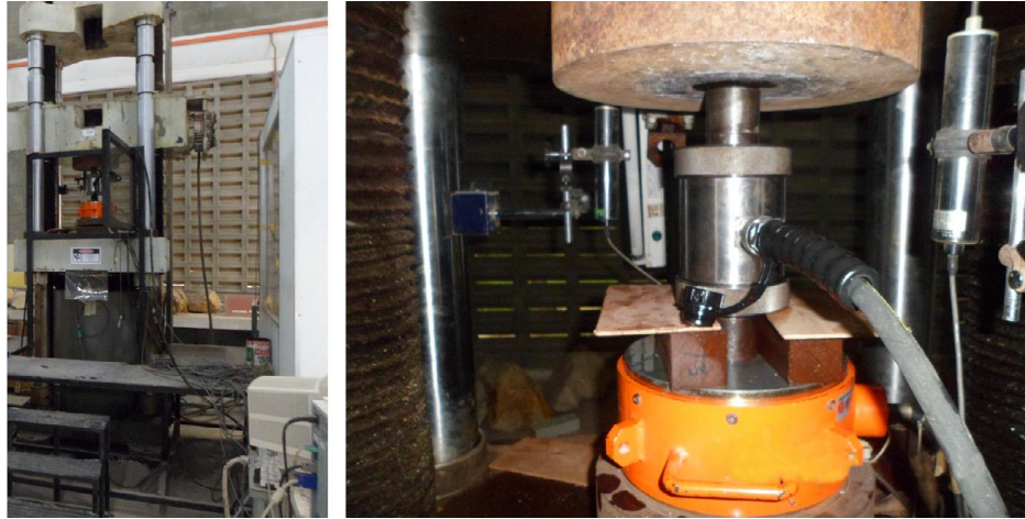
Fig. 4 Universal servo-controlled 3000 KN testing machine (Jahed Armaghani et al. 2014)
