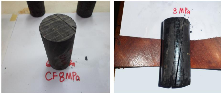
Fig. 5 Specimen with 8 MPa cell pressure before and after test conduction (Jahed Armaghani et al. 2014)
