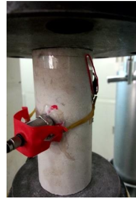
Fig. 2 The installation of AE probe
