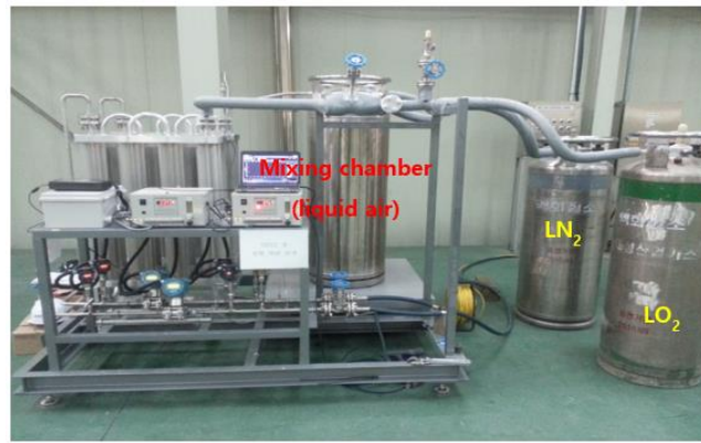
Fig. 2 Overview of apparatus for producing liquid air
