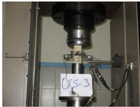
Fig. 3 (a) Schematic view of specimen and flaw geometry parameters, 2a: flaw length, "A": flaw aperture and \theta : flaw inclination and (b) Loading apparatus
