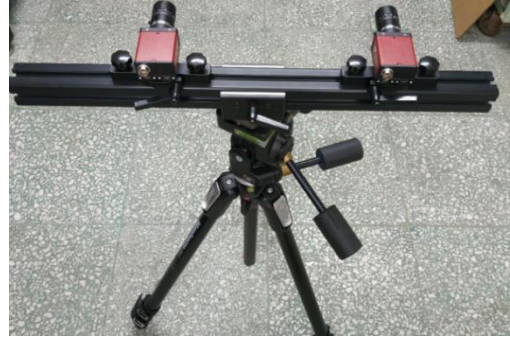
Fig. 9 Non-contact whole field strain measurement system
