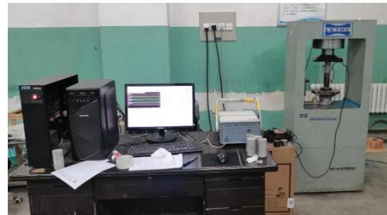
Fig. 2 Rock mechanics testing machine
