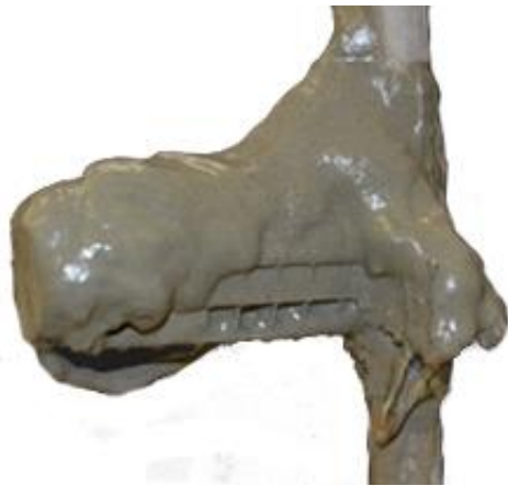
Fig. 11 Accumulation of denser backfill on the cages and top face of the vertical stress sensor near the center of the column
